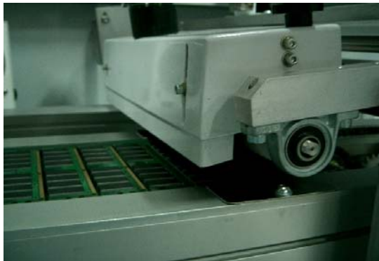
System here is used for brushing components after laser marking.
